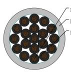
Bare copper conductor LSOH thermoplastic compound outer jacket HEPR insulation
